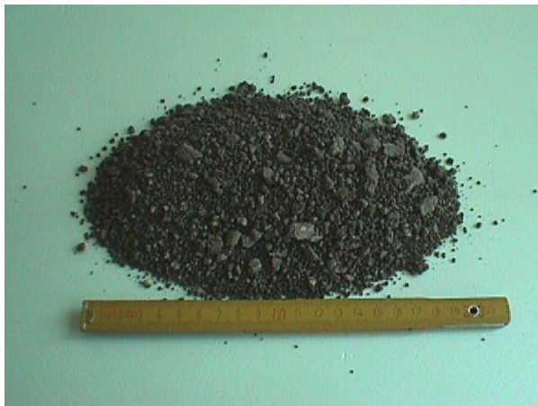
Granular pre-product (Sludge + P.C.) after hardening
